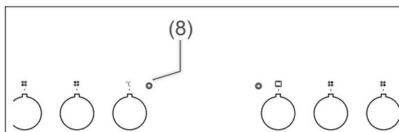
The red oven light (8) will illuminate as soon as you have selected a heating method and set the temperature. It will light up while the oven is heating up and/or re-heating. Once it goes out, the set oven temperature has been reached.
