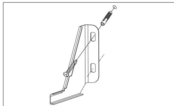
8. For solid walls: Place the supplied dowels into the holes. Screw the tilt protection tight with the supplied screws. For drywalls: Obtain suitable special dowels for the wall. If necessary, consult a professional.
