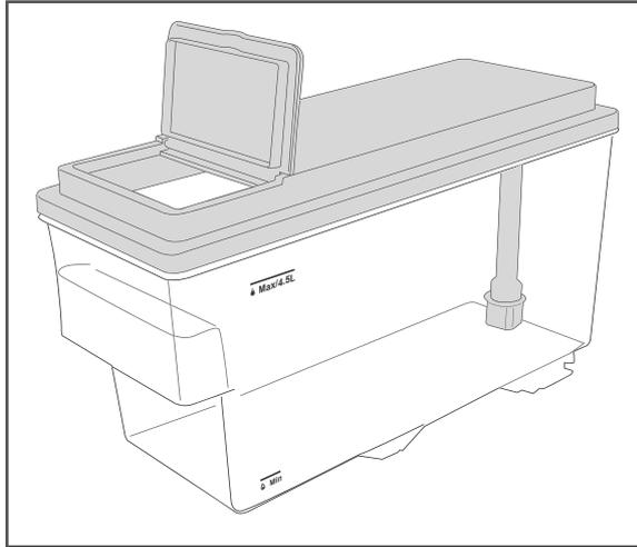
1. Open the lid and fill the water tank (13) with cold, fresh tap water so that the water level is above the "Min" mark but below the "Max" mark (4.5 L).
