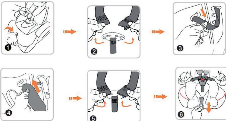
1. Press the harness adjuster lever with one hand, then pull the shoulder belt harness forward using the other hand to loosen it (fig.1).
