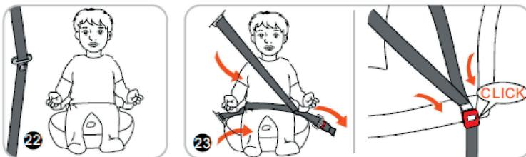
3. Place the child car seat on the passenger seat ensuring that it is firmly pressed against the vehicle seat (fig.22).
