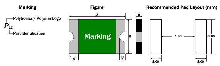
Note: Polystar is Polytronics's manufacturing site in China. The Polystar ID marking shall appear on smallest package.
