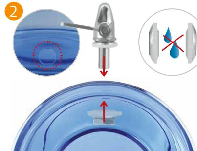
Mount the water tap with two seals (dry) on the inside and outside of the tank.
