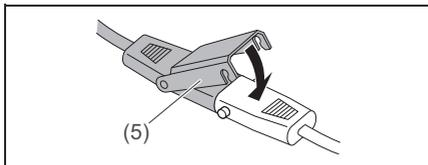
2. Fold the latch (5) down to securely lock the plug connection.
