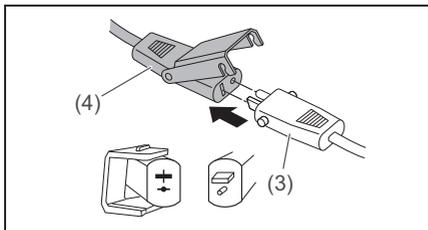
1. Insert the plug (3) into the jack (4). The form of the contacts prevents any reversal of polarity.
