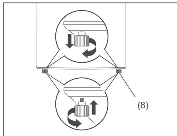
2. Level out any unevenness on the ground using the two front screw feet (8).
