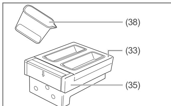
2. Fill the measuring cup (38) for each ice cube tray (34) up to the 55 ml mark with cold, fresh tap water.
