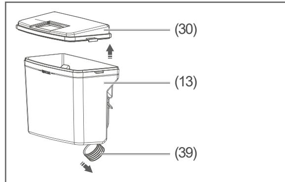
2. Remove the lid (30) and the sealing ring (39) of the water tank (13).
