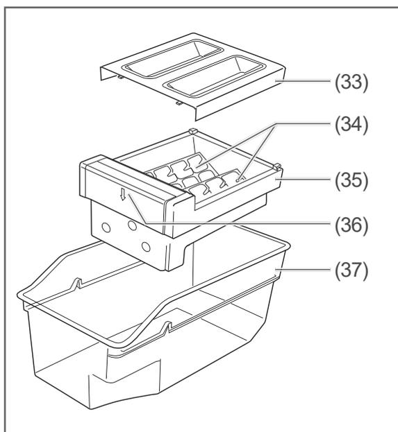
Your appliance has an ice cube maker (35) with a lid (33), two ice cube trays (34) and an ice cube collecting container (37). You can remove the ice cubes from the ice cube trays using the ejector (36).
