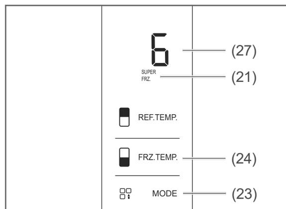
2. Press the FRZ.TEMP. button for 3 seconds.
