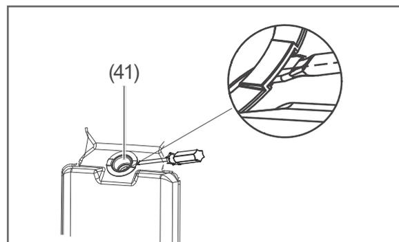
1. Lift the valve of the water dispenser a little with the help of a thin, flat tool.
