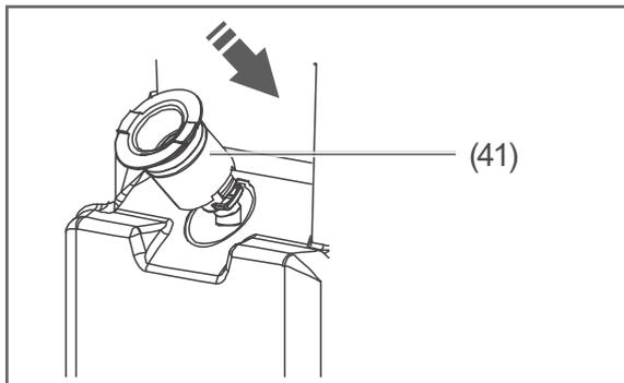
4. Press the water valve (41) back into the left fridge door, until you hear a click. To do this, position the valve at the slit.
