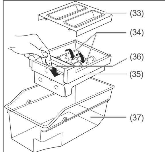
2. Press the ejector (36) of the ice cube maker firmly downwards in the direction of the arrow. Make sure that you press the ejector all the way down. The ice cube trays (34) turn. The ice cubes will fall into the ice cube collection container (37).
