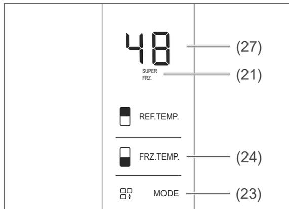
3. To set the duration of the SUPER FRZ. mode to 48 hours, press again the FRZ. TEMP. button
