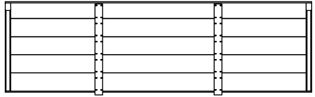
RP2 | ROOF PANEL - W2A03280 (x2) | 1 3/4"x16 1/4"x53 3/4" (45x417x1366)
