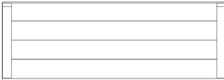
RP3 | PEAK ROOF PANEL - W2A02626 (2) | 1 5/8"x20 5/8"x59" (42x524x1499)
