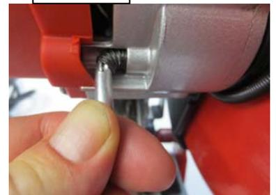
While the shaft lock is pressed solve with an Allen wrench size **8** by turning the screw counterclockwise **Fig. O**
