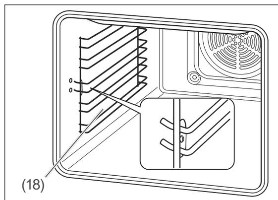
2. To remove the baking tray guides (18), first pull out the front holder on the front side, where the two hooks with the welded plates are. Then pull out the rear mount of the baking tray guides.
