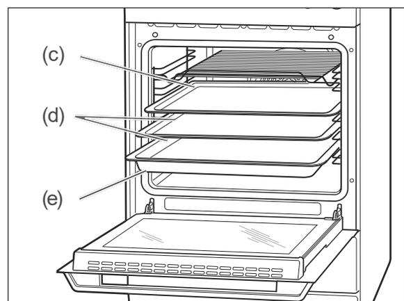
The supplied baking trays (d) and the dripping pan (e) have an angled edge. Please ensure that this edge is facing forward on being placed in the oven. The grilling rack (c) must be inserted as shown.
