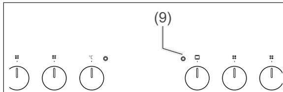
The yellow power indicator light (9) is illuminated as soon as at least one of the cooking zones or the oven is switched on. It will switch off again when **all** of the cooking zones **and** the oven are switched off.
