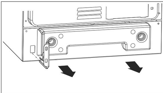
9. Slide the cooker into place and check that the tilt protection prevents the cooker from tipping forward.
