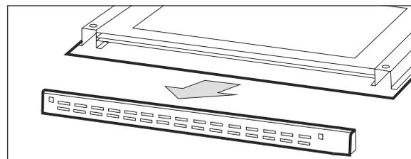
3. Carefully removed the metal grid.
