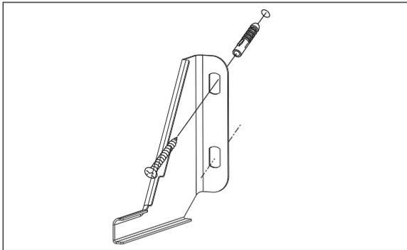
8. For solid walls: Place the supplied dowels into the holes. Screw the tilt protection tight with the supplied screws.
