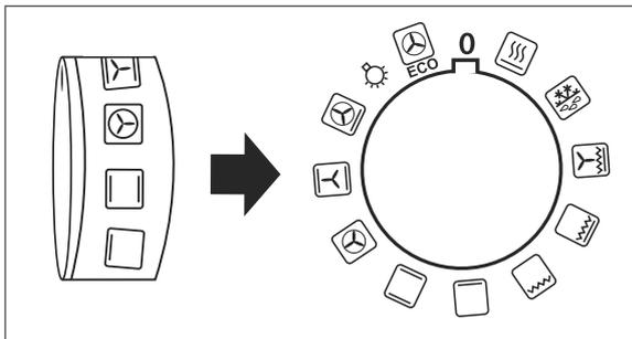
Use the oven dial to switch on the oven and select the heating method. The oven light will turn on.
