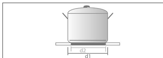
The d1 diameter is always provided as a pan and pot size. d2 base diameter is always around 2 cm smaller. Pots that are too big can cause paintwork damage.
