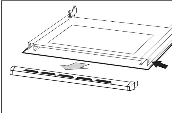
1. Carefully remove the grid cover by pushing down on the latches on the sides.
