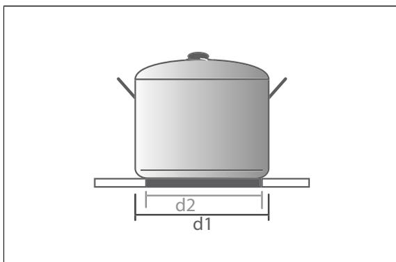
The diameter  $d_1$  is always given as the size of the pot or pan. Base diameter  $d_2$  is always around 2 cm smaller. Pots that are too big can damage paintwork.
