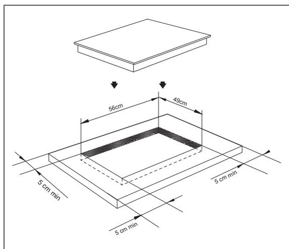
4. Make sure that there is a recess in the work surface corresponding to the dimensions shown in the illustration. The space above the hob should be at least 76 cm.
