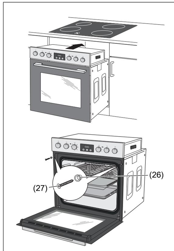
5. When the oven is correctly aligned, open the oven door and screw it firmly to the built-in cabinet using the enclosed assembly material (26), (27).
