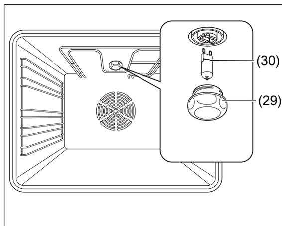
3. Unscrew the glass cover (29) anticlockwise and remove it.
