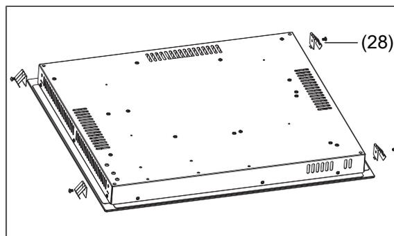
5. Attach the retaining clips to the hob using the screws (28).
