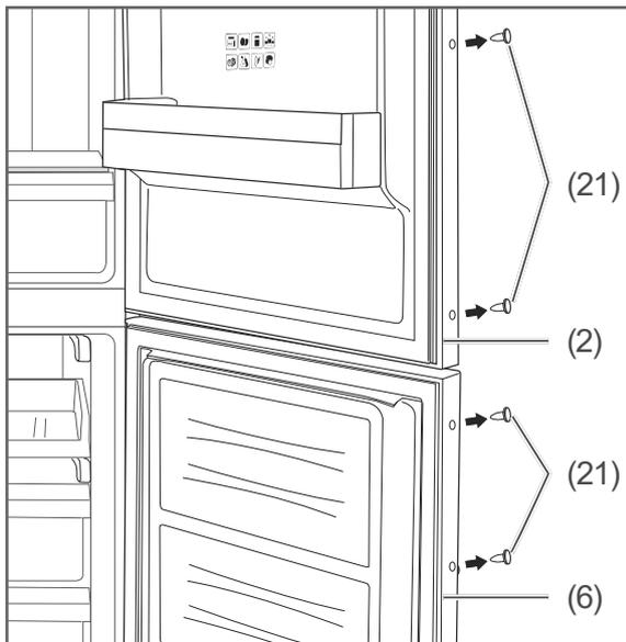
1. Lift out the blind plugs (21) from the side of the appliance doors (2) and (6).
