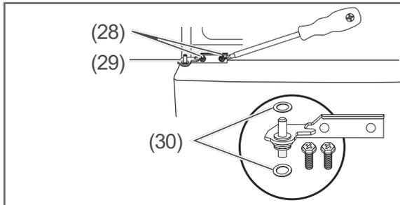
5. Use the screws (28) to attach the middle hinge (29).
