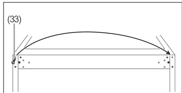
10. Loosen the screw (33) and place it back on the opposite side.
