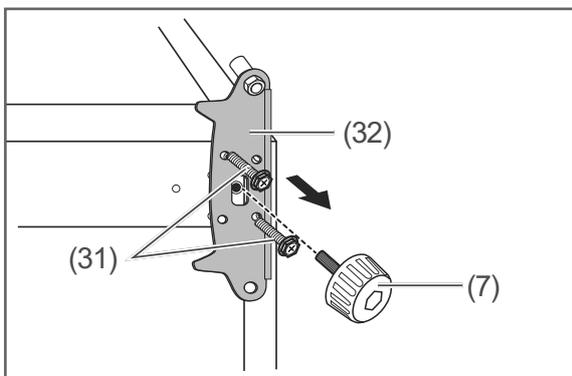
8. Loosen the screws (31) on the lower hinge (32), unscrew the right screw foot (7), and remove the hinge.
