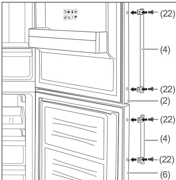
2. Use the included screws (22) to attach the longer door handle (4) to the fridge door (2), and the shorter door handle to the freezer door (6).
