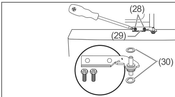
5. Loosen the screws (28) on the middle hinge (29) and remove the middle hinge. Retain the two washers (30).
