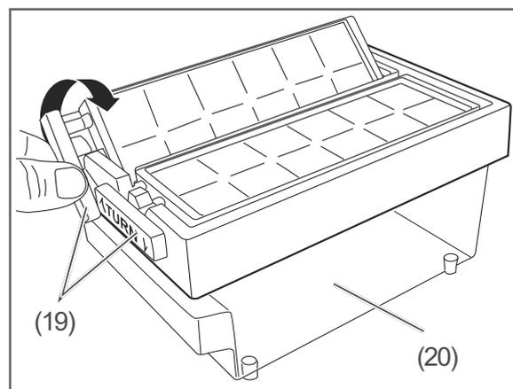
2. To remove the ice cubes, twist the levers (19) clockwise. This will turn over and also slightly twist the ice cube trays (17), causing the ice cubes to fall into the storage container (20).
