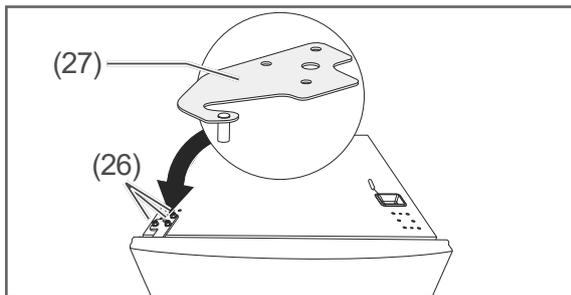
7. Attach the upper hinge (27) and fasten it using the screws (26) provided.
