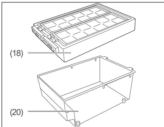
3. Remove the ice maker (18) from the storage container (20), and take out the ice cubes. You should ideally use an ice scoop (not included) to do this in order to avoid freeze burn.
