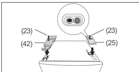
8. Fit the left hinge cover (42) and fasten it using a screw (23).
