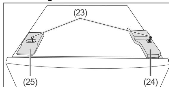
1. Use the cross-tip screwdriver to loosen the screws (23) on the covers (24) and (25).
