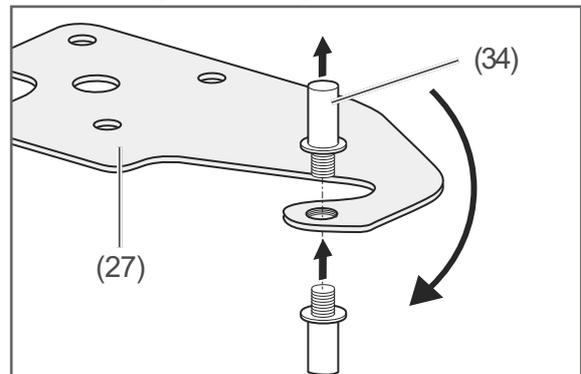
1. Unscrew the hinge bolt (34) of the upper hinge (27) (ideally using a pair of pliers) and screw it back in on the opposite side.
