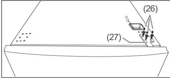
3. Loosen the screws (26) on the upper hinge (27) and remove the hinge.
