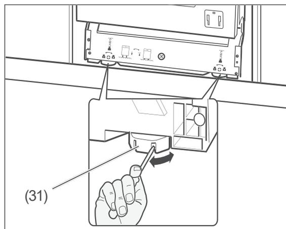
8. To position the dishwasher so that it is level, the two front adjustable feet (31) and the back foot on the appliance can be adjusted by up to 50 mm.
