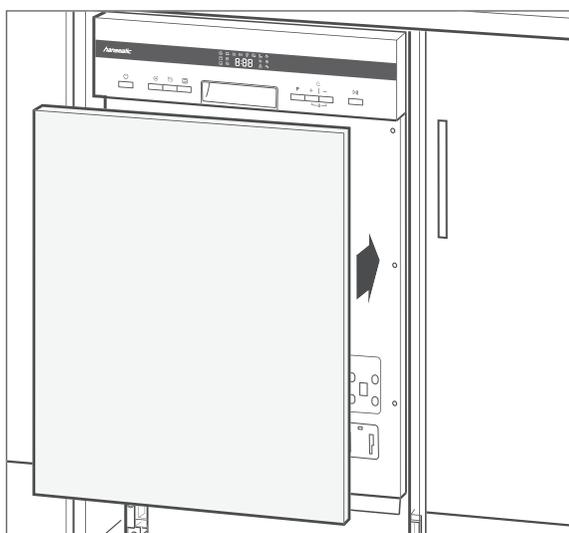
16. Fix the front panel to the dishwasher door using the hook-and-loop straps (40), hold it firmly, and open the door carefully.
