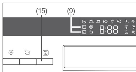
If only one of the two dish racks is loaded, you should deactivate the spraying arm which you do not require.
