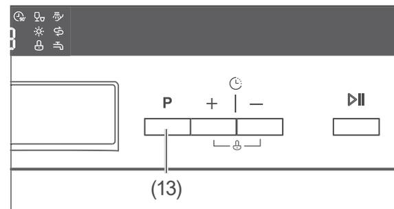
2. Press and hold the **P** button (13) for as long as required until the current water hardness is shown on the display: H 1 to H 6.
