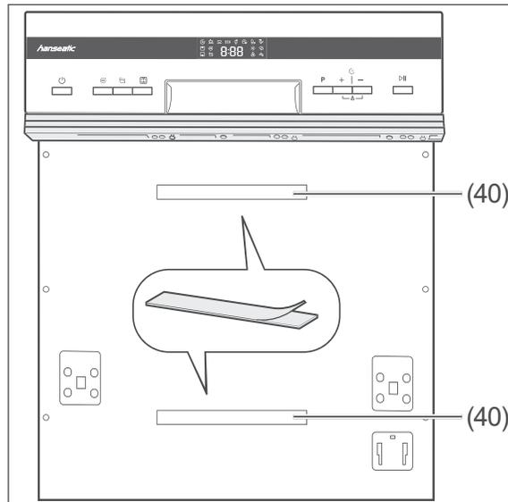
9. With the protective film removed, affix the hook-and-loop straps to the middle of the recessed areas on the dishwasher door.
