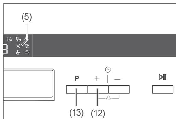
2. Press the **P** button (13) for 5 seconds within 60 seconds of switching on.
