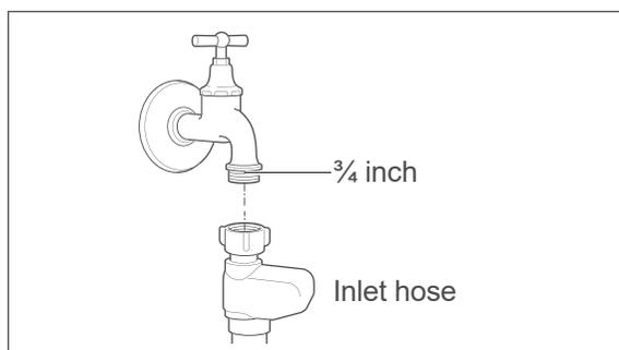
For water supply, you need a water tap with a  $\frac{3}{4}$  inch screw connector.
