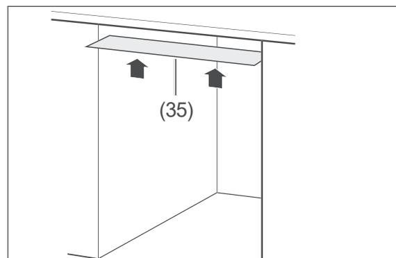
3. Affix the enclosed condensation-protective film (35) to the bottom of the work surface. In this way, you will avoid damage to the worktop caused by hot steam emitted from the dishwasher when the appliance door is left open.
