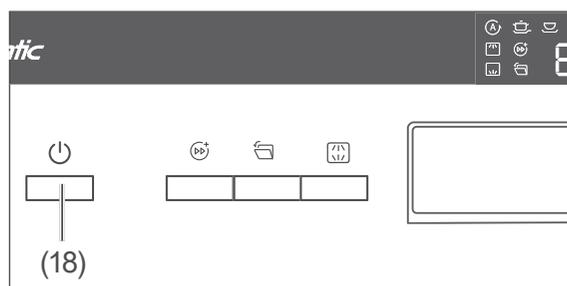
3. If the dishwasher is switched on, switch it off with the  $\odot$  button (18).
