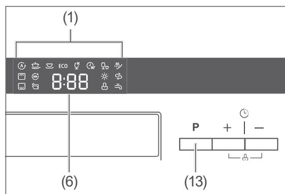
2. Press the **P** button (13) as often as required until the display shows the desired programme indicator (1) and the programme duration (6).
