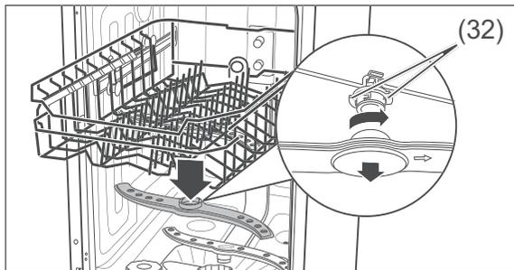
3. The upper spraying arm is affixed using a bayonet closure. To remove the spraying arm, hold the two serrated bayonet grips (32) still and turn the spraying arm clockwise.
