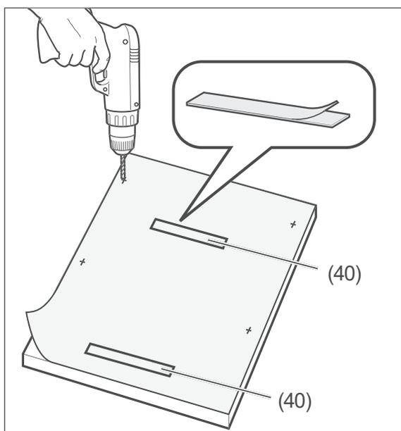
12. Lay the enclosed drilling template on the **back** of the front panel in such a way that the drilling template and the front panel are flush at the top.
