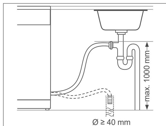
You can connect the end of the outlet hose in two different ways:
