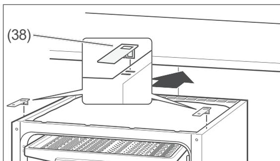
4. Insert the two mounting brackets (38) into the front slots on the top of the dishwasher so that you can screw the dishwasher to the worktop subsequently.
