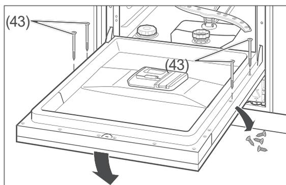
17. Remove the 4 screws from the inside of the door. Screw the front panel in place at these positions using the 4 enclosed screws (43).
