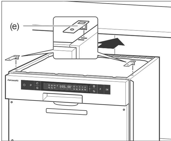
4. Insert the two mounting brackets (e) into the front slots on the top of the dishwasher so that you can screw the dishwasher to the worktop subsequently.
