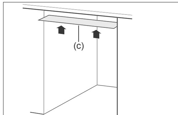
3. Affix the enclosed protective film (c) to the bottom of the work surface. In this way, you will avoid damage to the work surface as a result of hot steam which may be emitted from the dishwasher if the dishwasher door is left open.
