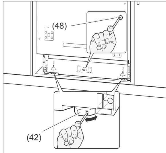
8. To position the dishwasher so that it is level, the two front adjustable feet (42) and the back foot on the appliance can be adjusted by up to 50 mm.
