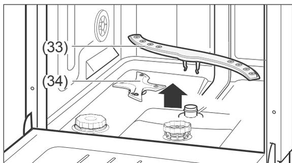
2. Turn the lower spraying arm (33) upward and outwards.
