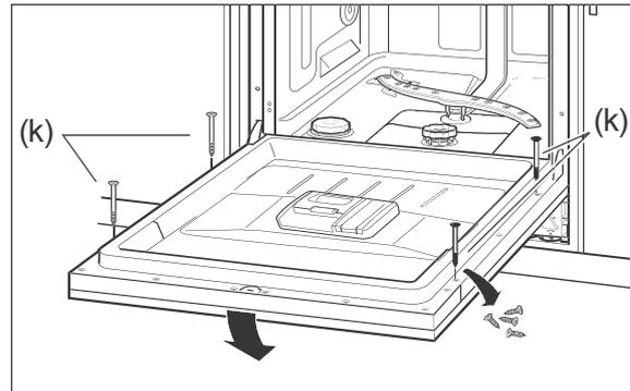
17. Remove the 4 screws from the inside of the dishwasher door. Screw the front panel in place at these positions using the 4 enclosed countersunk screws (k). The front panel has been successfully mounted.
