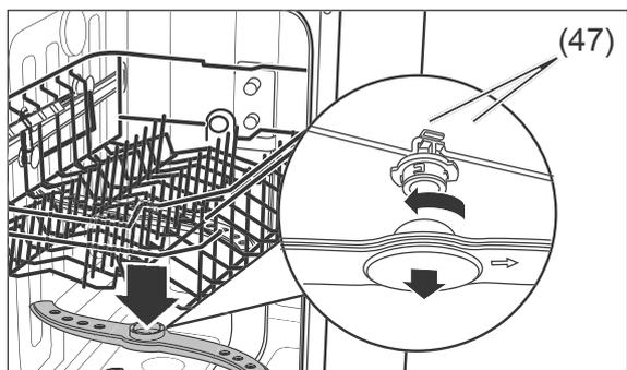
3. The upper spraying arm is affixed using a bayonet closure. To remove the spraying arm, hold the two serrated bayonet grips (47) still and turn the spraying arm clockwise.
