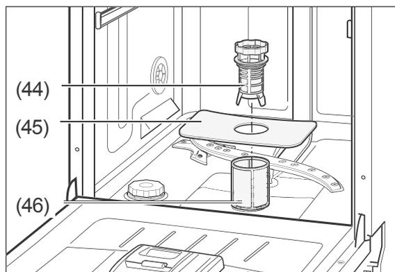
Check the coarse filter (44), the main filter (45) and the fine filter (46) after each rinse cycle and remove food residues and foreign bodies if necessary.
