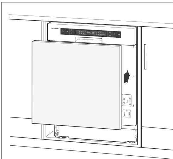
16. Attach the front panel to the door of the dishwasher using the velcro straps (h), hold the panel in place, and carefully open the dishwasher door.
