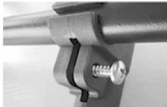
At the lower end of the telescopic supports, there is a hexagonal screw fitted, turn this until it sticks out by about 20 - 30 mm and fit the rubber feet with the small diameter onto the ends.
