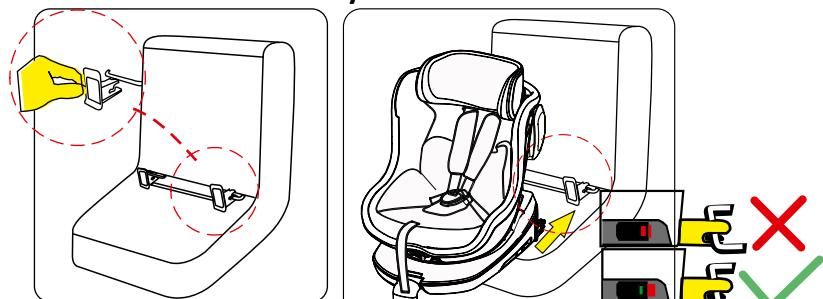
Step 1: Install ISOFIX guide sleeves to ISOFIX lower anchorages.
