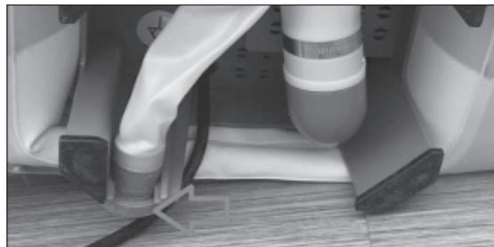
3. Screw the filter cartridge on to the water inlet of the SPA wall by turning it clockwise and place the cover on the filter cartridge. This cover retains hair and coarse dirt particles that would otherwise contaminate your filter cartridge more quickly.
