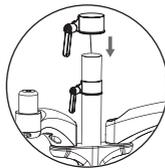
**Insert steel fastener to the steel pipe.**
