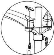
**Insert the screw through the hole from supporting part to the decorative cap.**
