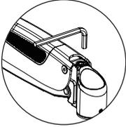
**NOTE:** Turn clockwise to reduce tension for lighter monitors and counter-clockwise to increase tension for heavier monitors. Keep adjusting until monitor can keep still at any position.
