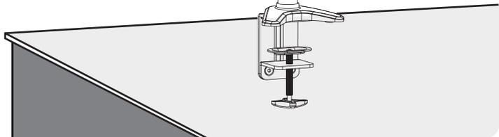
**Tighten clamp using clamp screw until mount is securely fastened to desk.**
