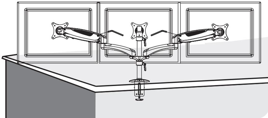
**Use a hex wrench to adjust the height tension of the gas spring arm, to keep different weight of monitors still at any position.**
