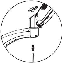
Insert the screw through the hole from extension arm to the decorative cap.
