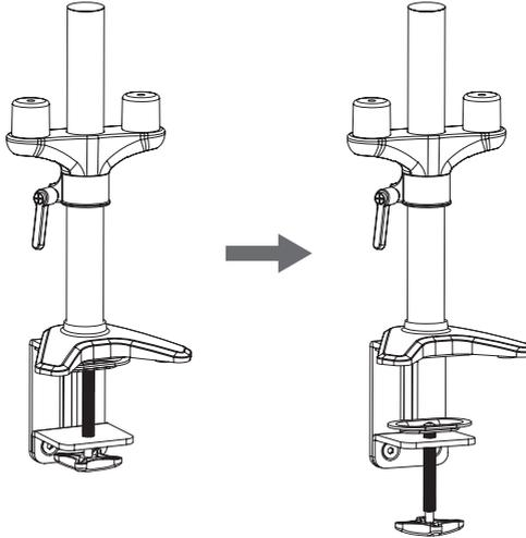
**Loosen clamp screw until enough space is left for the edge of the desk.**
