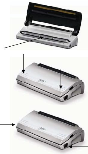
**Step 1:** Open the lid and place an open side of the bag in the vacuum chamber- with the smooth side up.
