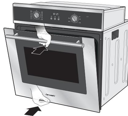
1. Hold the door on an angle using both hands.
