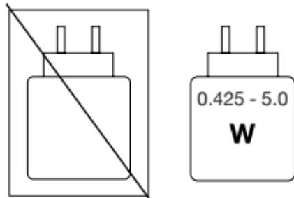
The power delivered by the charger must be between min 0.425 Watts required by the radio equipment, and max 5.0 Watts in order to achieve the maximum charging speed.
