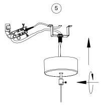
Insert the bulb & screw the lamp.
