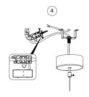
Connect the 3 wires & Apply the screws
