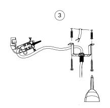
Unscrew the screw of the bracket
