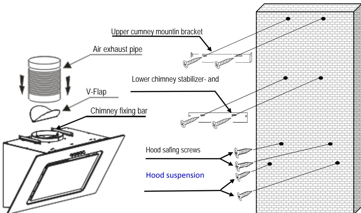
\*The screws installed should leave for 3-5mm out of the wall to hang the hood on them
