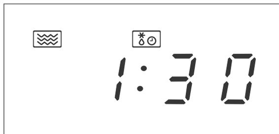
3. Turn the control dial (3) to set the desired defrosting duration (between 5 seconds and 95 minutes).
