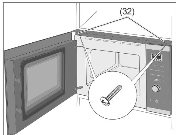
2. Screw the appliance into the drilled holes (32) using the screws provided and a Phillips screwdriver.
