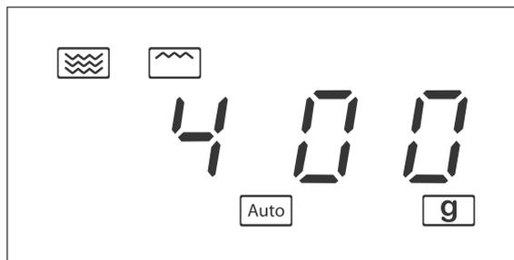
9. Press the 'START / +30Sek. / Bestätigen' sensor (27) to confirm the weight. The appliance starts. The ventilator starts. The light in the cooking chamber switches on. The glass rotary plate starts to turn. On the display, the pre-programmed time will now count down. The symbol of the selected programme flashes. Five beeps will sound once the cooking time has expired. The appliance switches off. The display now again shows the time.
