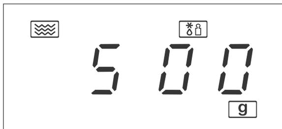
3. Turn the control dial (3) in order to enter the weight of the dish (between 100 g and 2000 g, in 100 g steps).
