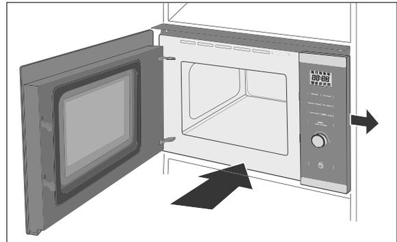
1. Push the appliance into the installation compartment until the front panel meets the frame of the installation compartment.
