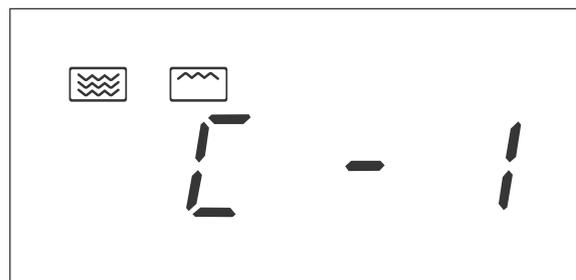
2. Press the 'Grill / Kombi.' sensor (24) once. Turn the control dial (3) or press the 'Grill / Kombi.' (24) repeatedly until - 1 or - 2 flashes on the display, and the symbols (13) and (14) appear.
