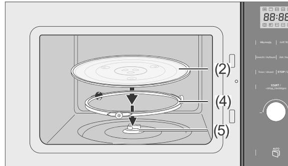
1. If necessary, place the turntable drive (5) in the central recess.
