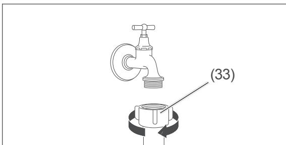
2. Secure the other end on the water inlet hose to the tap by hand. Then turn the union nut (33) clockwise.
