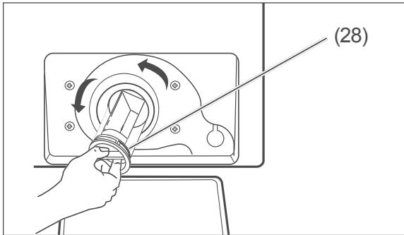
4. Place a suitable collecting container underneath the lint trap (28).
