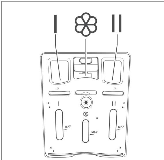
The dispenser is located on the inside of the appliance lid and has (16) three compartments:
