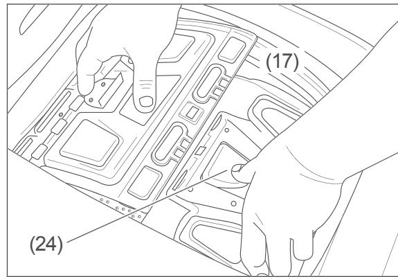
3. To open the washing drum, (17) press the plastic tab(24) down slightly on the smaller section of the lid until the locking hooks disengage.
