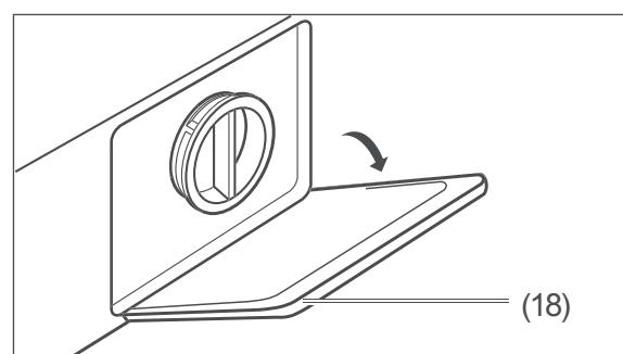
3. Carefully open the shutter (18) of the lint trap with a flat object, such as with a flat-tip screwdriver.
