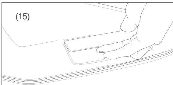
1. Open the appliance lid (15) by reaching under the handle and folding the lid upwards.
