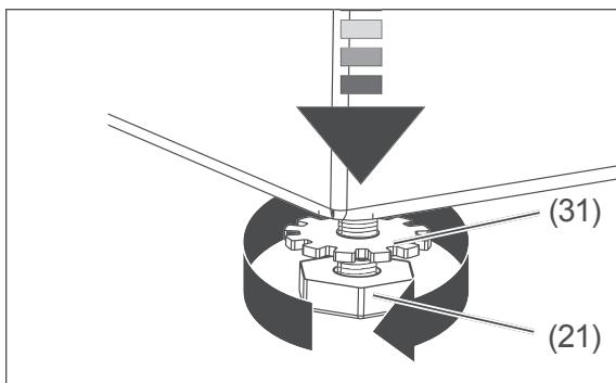
1. Loosen the lock nut (31) of one of the screw-on feet (21) underneath the appliance.
