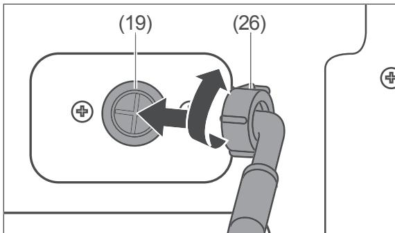
5. Unscrew the water inlet hose from the appliance.
