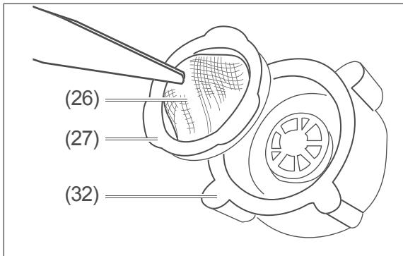
6. Use tweezers or a pair of pliers to pull the filter (26) with gasket (27) out of the union nut (32). Rinse the filter under fresh water and clean with a small, soft brush if necessary.
