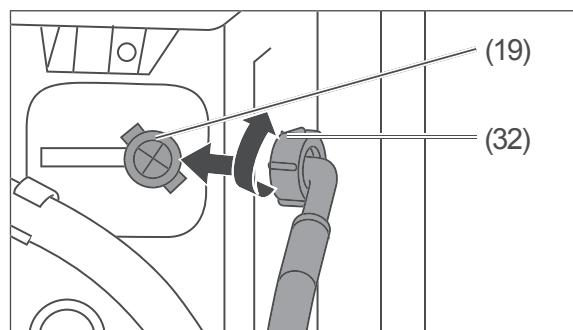
1. Screw the enclosed water inlet hose onto the connection (19) by hand. To do so, turn the union nut (32) clockwise.
