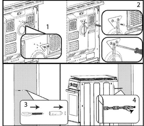
**i** Stability chain to be as short as practicable to avoid oven tilting forward and diagonal to avoid oven side tilting.
