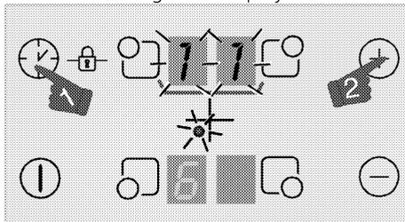
**i** Right rear and left rear cooking zone displays serve as timer display when the timer is active.
