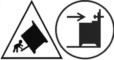
**Warning:** In order to prevent tipping of the appliance, this stabilizing means must be installed. Refer to the instructions for installation.
