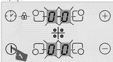
**i** If no operation is performed within 20 seconds, the hob will automatically return to Standby mode.
