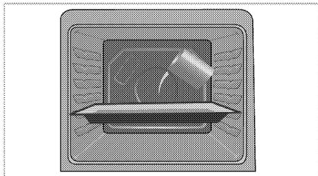
3. Set the oven to easy steam cleaning mode and run at 100°C for 25 minutes.
