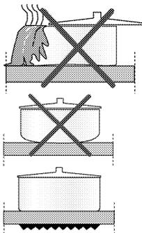
Spills may damage the glass ceramic surface and cause fire.
