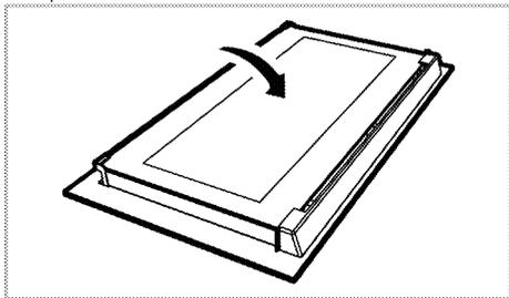
2. Pull towards yourself and remove the plastic part installed to upper section of the front door.
