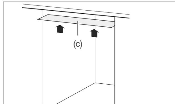
3. Affix the condensation protection film supplied (c) to the underside of the worktop. In this way, you will avoid damage to the work surface as a result of hot steam which may be emitted from the dishwasher if the dishwasher door is left open.
