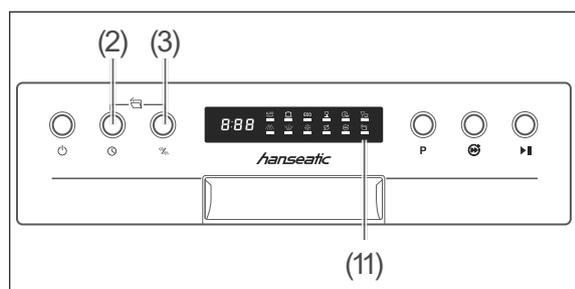
The “Automatic door opening” function is activated as standard. The appliance door opens automatically during the drying phase of the dishwashing programme and remains open.
