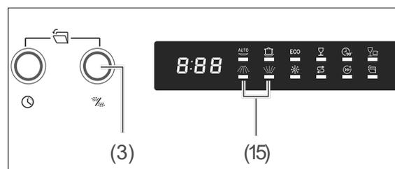
If only one of the two dish racks is loaded, you should deactivate the spraying arm which you do not require.
