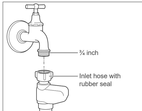
You will require a valve with a  $\frac{3}{4}$ -inch screw connector for the water supply.
