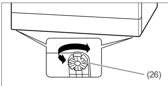
3. In order to equalise unevenness in the floor and set up the dishwasher on a level horizontal base, you can screw the four appliance feet (26) in or out. There are slots in the appliance feet around the circumference. Insert a screwdriver and turn the appliance foot.
