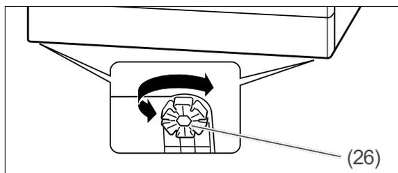
5. In order to equalise unevenness in the floor and set up the dishwasher on a level horizontal base, you can screw the four appliance feet (26) in or out. There are slots in the appliance feet around the circumference. Insert a screwdriver and turn the appliance foot.
