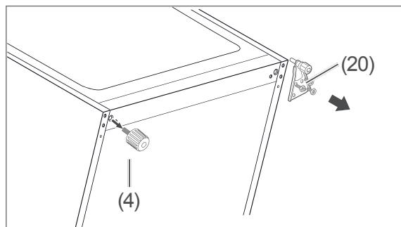
6. Tilt the unit slightly backwards against a wall so that the lower hinge (20) is accessible.
