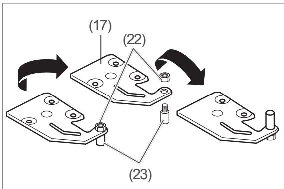
1. Using pliers, loosen the nut (22) on the upper hinge (17), unscrew the hinge bolt (23) of the upper hinge (17) and screw it back in on the other side of the hinge plate.
