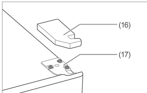
2. Using a Phillips screwdriver, lift out the protective cover (16) of the upper hinge (17).
