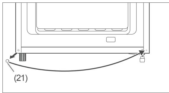
9. Remove the protective cap (21), and place it back onto the screw on the opposite side.
