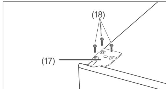
3. Replace the upper hinge (17) and screw it tight using the screws (18) provided. Check whether the doors are easy to open and close.
