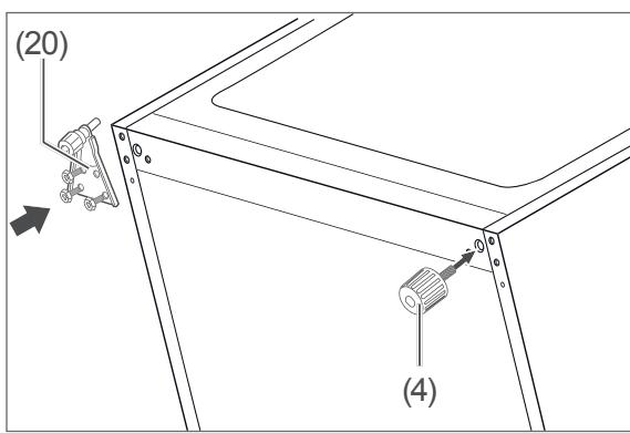
1. Reinsert the lower hinge (20) and the screw foot (4) into the new position.
