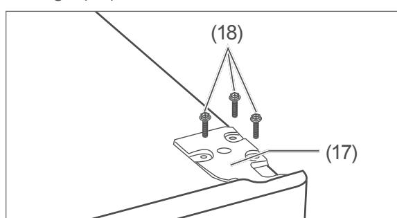
3. Unscrew the 3 screws (18) on the upper hinge (17) and remove the hinge (17).
