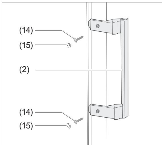
4. Secure the door handle (2) to the door using the screws provided (14).
