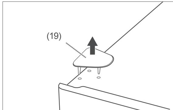
4. Using a flathead screwdriver, lift out the cover (19) on the opposite side.
