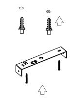
2. Align, mark and drill holes to apply the base on the ceiling
