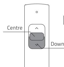
**11.1** Simultaneously hold the **centre** and the **down** button until the blind stops stepping and starts stepping again.
