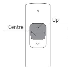
**9.1** Simultaneously hold the **centre** and the **up** button until the blind stops stepping and starts stepping again.
