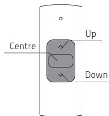
**i** **Remote control:** Press the **up** or **down** button to operate the blind. Press the **centre** button to stop the blind.
