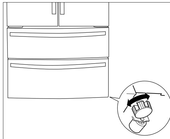
3. Screw in or unscrew the feet until the combination fridge-freezer is vertically aligned.
