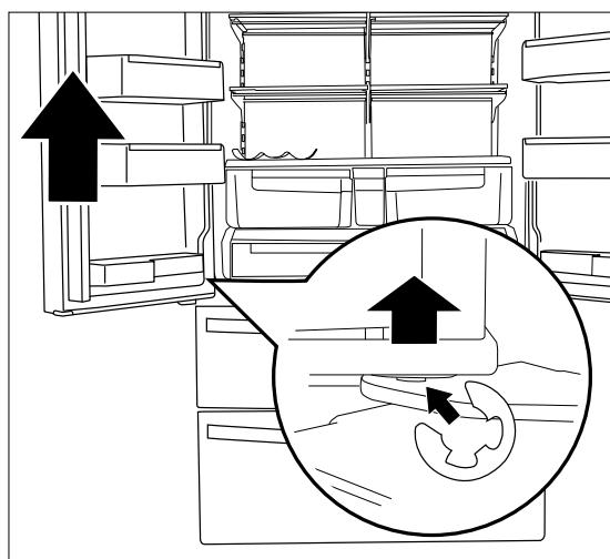
1. Open the door and lift it up. This will create a gap between the bottom door hinge and the door.
