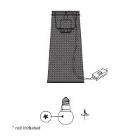
1. Install the bulb from the bottom of the base
