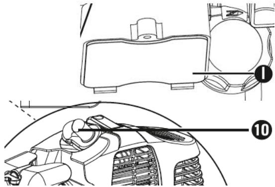
Electrode gap = 0.6 mm (distance between the electrodes between which the ignition spark is generated). Check the spark plug for contamination after the first 10 hours of operation and clean it with a copper wire brush if required. Afterwards, service the spark plug after every 25 hours of operation.
