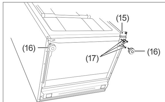
8. Tip the appliance back as far as possible (45° max.) in such a way that the front feet (16) of the appliance and the lower hinge plate (15) are easy to reach.
