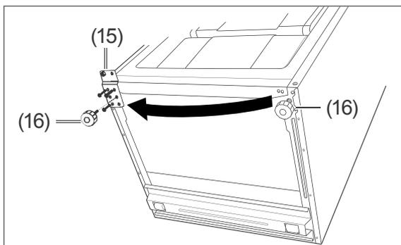
13. Screw the hinge plate (15) back onto the opposite side.
