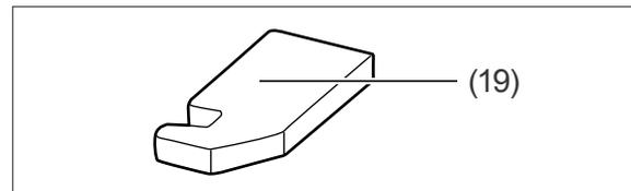
24. Press the hinge faceplate (19) onto the hinge plate and the covering plate into the holes on the opposite side.
