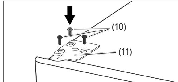
22. Place the upper hinge plate (11) on the fridge door and then screw it tight using the three screws (10).
