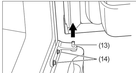
5. Open the fridge door and lift it vertically upwards from the bolt on the middle hinge (13).
