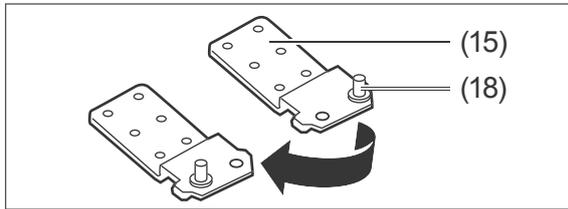
12. Replace the hinge bolt (18) as shown above.
