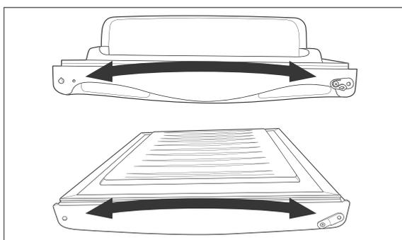
17. Unscrew the hinge bushings from the top of the fridge compartment door and on the bottom of the freezer door and screw them back on tightly on the opposite side.
