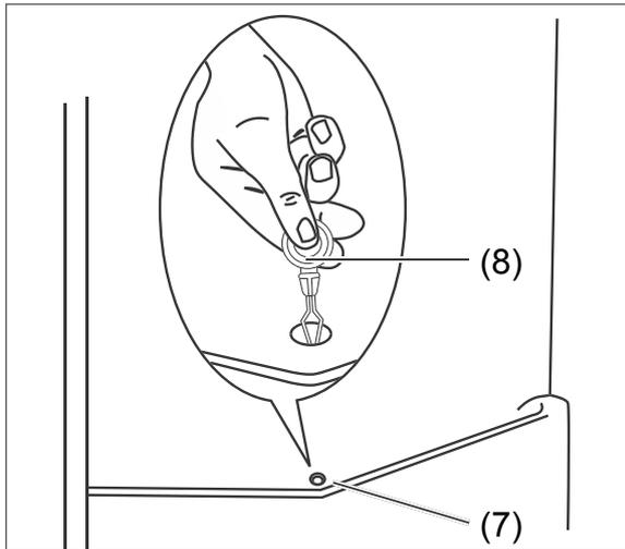
11. The defrost water drain (7) can be found on the rear wall of the fridge above the vegetable drawer. The cleaning tool (8) can be found in the opening of the defrost water drain. Use it to clean the defrost water drain.
