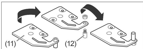
4. Unscrew the nuts from the hinge bolts using a size 10 spanner. Unscrew the hinge bolts (12) from the upper side of the hinge
