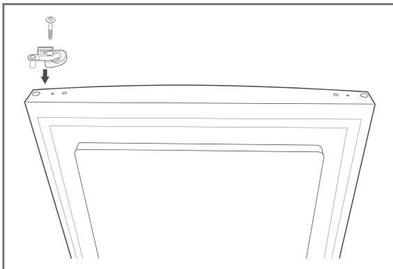
14. Insert the loose plastic insert supplied into the new hinge stop side and firmly screw in.
