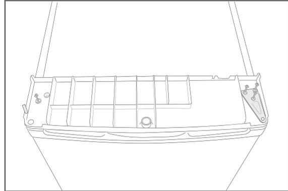
5. Unscrew the three fixing screws for the hinge plate and the one screw on the opposite side. To do this, use an 8 mm spanner or a cross-head screwdriver. Remove the hinge plate.
