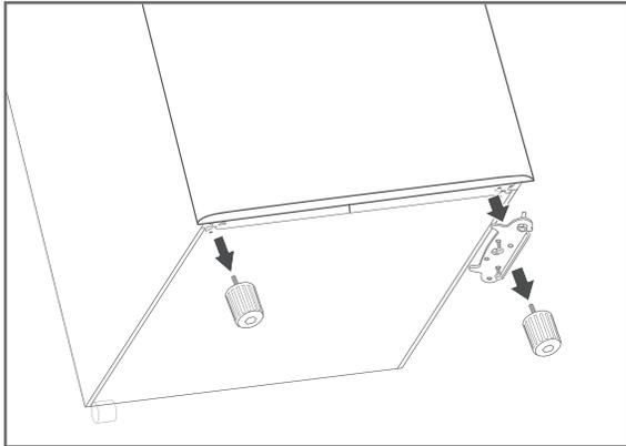
9. Tip the freezer backwards (maximum 45°) so that you can also move the lower door hinge.
