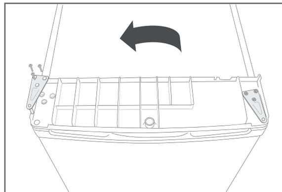
6. Screw the hinge plate as well as the one screw back onto the respective opposite side.
