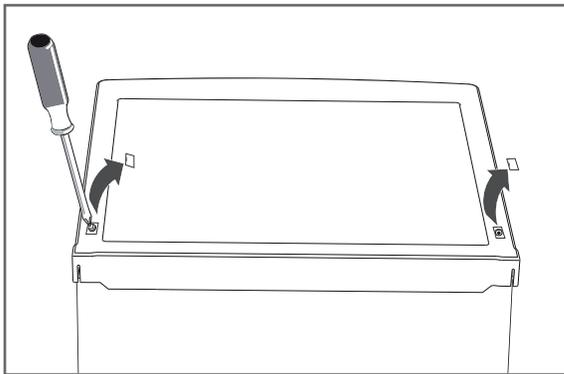
2. Loosen both screw covers on the top of the cover using a flat-head screwdriver.
