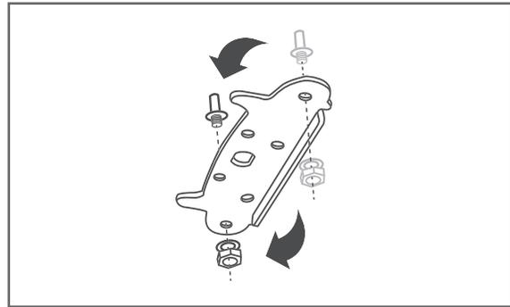
15. Turn the lower hinge plate. Loosen the hinge bolts with a 10 mm spanner. Loosen the nuts and reinsert the nuts and the hinge bolts from the other side. Move the screw (4) to the opposite side.
