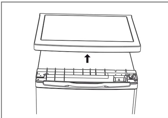
4. Lever out the two sides of the cover on the front slightly and lift the cover up. In doing so, ensure you do not damage the temperature controller (1).
