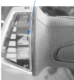
Shift grip marking 4 th gear
