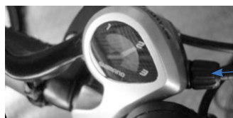
Knurled nut for fine adjustment
