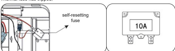
The vehicle is equipped with a self-resetting fuse. When the vehicle is overloaded or operated incorrectly, the self-resetting fuse will be cut off for 5 - 10 seconds before becoming operational again. The self-resetting fuse is under the seat. Cut off the power, follow these guidelines:
