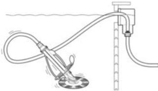
Set the multi-port in the FILTRATION position to vacuum the pool floor (e.g. with Ubbink PoolCleaner Auto, Art. No. 7500401). Connect the pool floor vacuum hose to the skimmer. The filtration group pump must be shut off.
