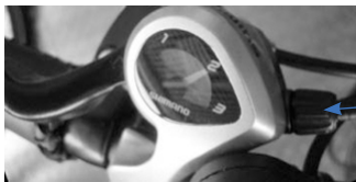
Knurled nut for fine adjustment
