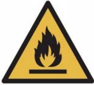
**EN WARNING: Risk of fire/flammable material.** The symbol indicates there is a risk of fire since flammable materials are used. Take care to avoid causing a fire by igniting flammable material.
