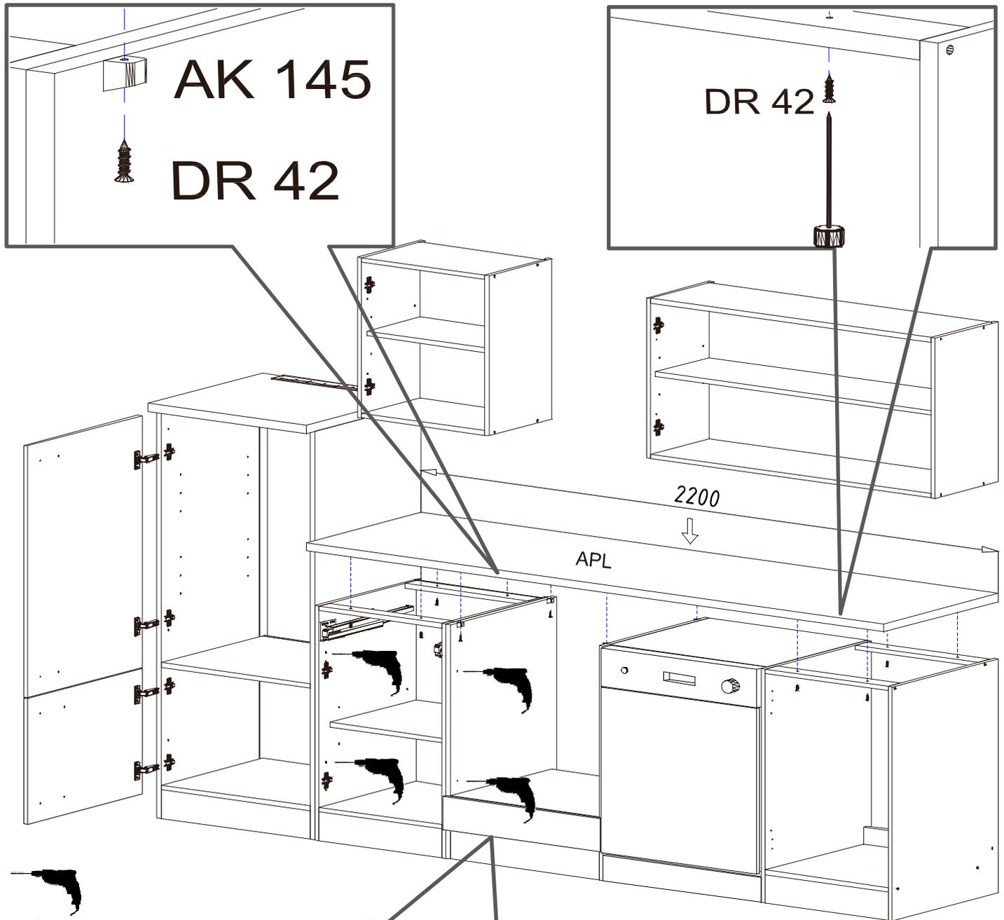
Mit  $\varnothing 5\text{mm}$  Bohrer durchbohren
