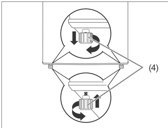
3. Level out any unevenness on the ground using the two front screw feet (4).
