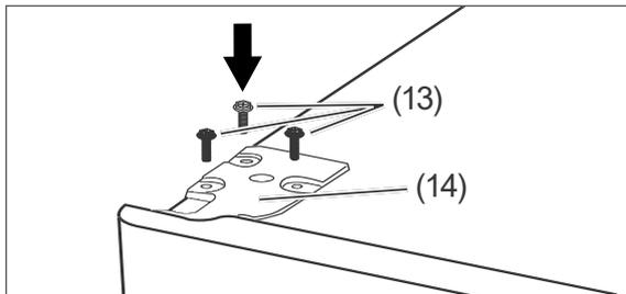
6. Place the upper hinge plate (14) on the fridge compartment door and then screw it tight using the three cross-headed screws (13).
