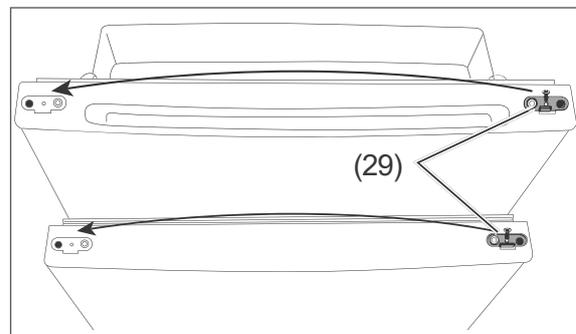
2. Unscrew the hinge bushings (29) from the top of the fridge compartment door and on the bottom of the freezer com-
