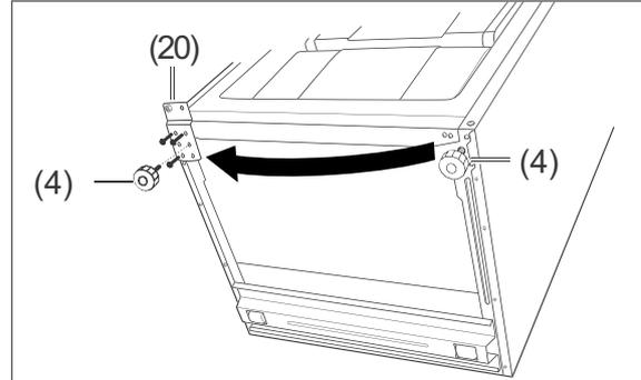
9. Screw the hinge plate (20) and the support plate back onto (26) the opposite side.
