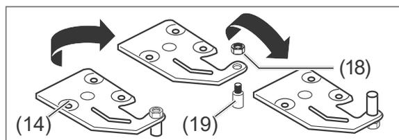
1. Unscrew the nuts (18) from the hinge bolts using a size 10 spanner (19). Unscrew the hinge bolts (19) from the upper side of the hinge faceplate (14) and re-screw them back onto the bottom. Rescrew the nuts tightly on to the hinge bolts.
