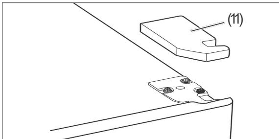
2. Carefully lift the hinge faceplate up (11) with the help of a flat-headed screwdriver.
