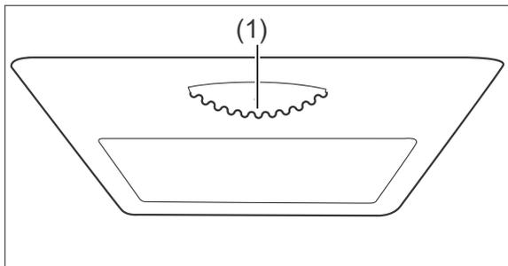
The temperature controller (1) can be used to switch the appliance on and off. It can be found at the top of the fridge compartment.
