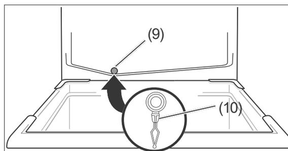
11. The defrost water drain (6) can be found on the reverse side of the refrigerator area above the vegetable drawer (9). The cleaning tool can be found in the opening to the thaw water drain (10). Use it to clean the thaw water drain.
