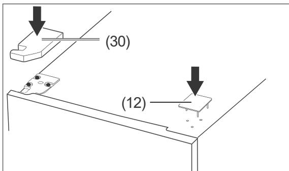
8. Press the hinge faceplate (30) onto the hinge plate and the covering plate (12) into the holes on the opposite side.
