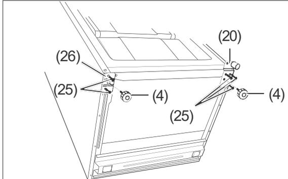
2. Tip the appliance back as far as possible (45° max.) in such a way that the front feet of the appliance (4) and the lower hinge plate (20) are easy to reach.
