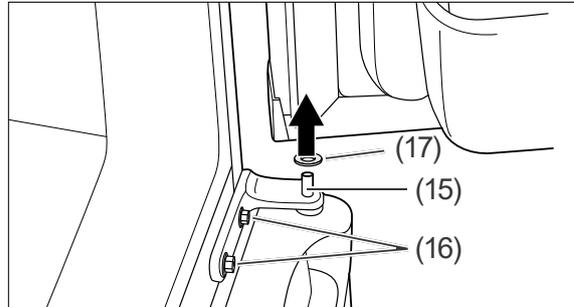
5. Open the fridge compartment door and lift it vertically upwards from the bolt on the middle hinge (15). Set the door aside.
