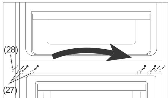
1. Remove the 3 blind plugs (27) and the decorative cap (28) on the left side in the area of the middle hinge and affix them in the corresponding positions on the opposite side.
