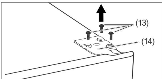
4. Loosen and remove the screws (13) and remove the upper hinge (14).
