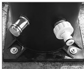
Discharge opening with a drain plug (left) Inlet fitting and hose connector (right)
