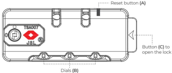
The lock is present at 0-0-0. Combination can be reset in the following way:
