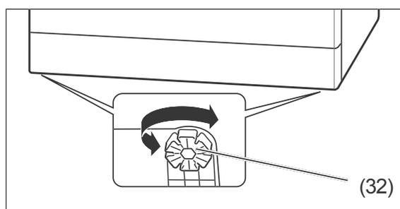
2. In order to compensate for uneven floor surfaces and set up the dishwasher on a level horizontal base, you can screw the four adjustable feet (32) in or out. The adjustable feet have slots around their circumference. Insert a screwdriver and turn the adjustable foot. Use a spirit level to set up the dishwasher.
