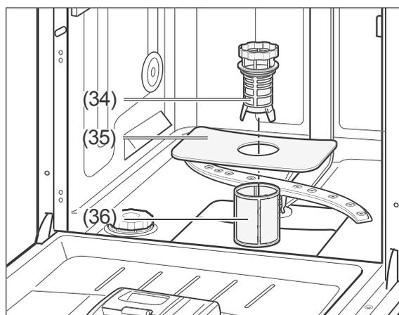
Check the coarse filter (34), the main filter (35) and the fine filter (36) after each rinse cycle and remove food residues and foreign bodies if necessary:
