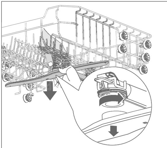
3. The upper spraying arm is affixed using a bayonet closure. Hold the two toothed bayonet handles firmly, turn them clockwise and remove the spraying arm.
