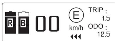
Press the power switch of the board, the board indicator will be turned on, and the remote will show speed, battery, mode and other information.
