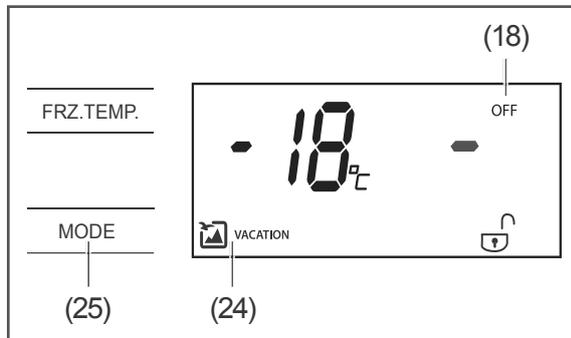
You can switch off the fridge compartment (e.g. while on holiday) without interrupting the power supply. The freezer compartment will stay cold.
