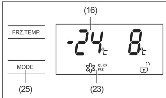
Select the setting (23) QUICKFRZ. “Quick freezing” to pre-chill the freezer compartment before storing food and to freeze fresh food.
