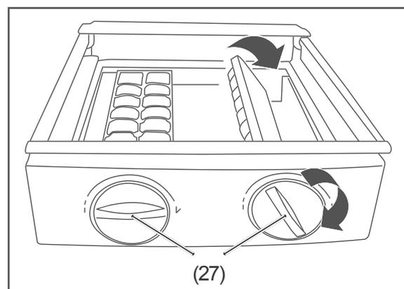
4. To loosen the ice cubes, turn the knobs (27) clockwise halfway. The ice trays will bend slightly, and the ice cubes will fall into the ice cube drawer (10).
