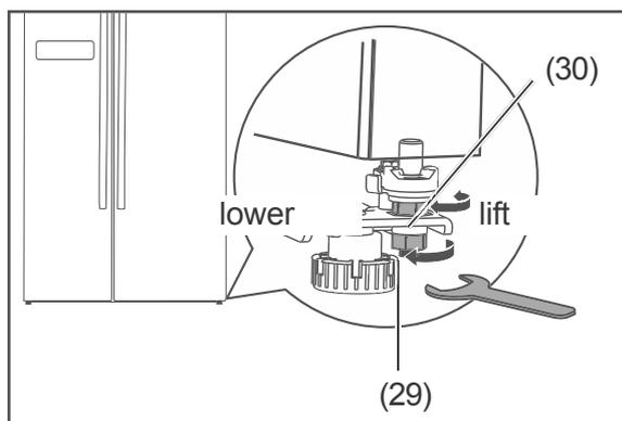
2. Turn the locknut (29) two full rotations clockwise to loosen it. Use the spanner supplied to do this.
