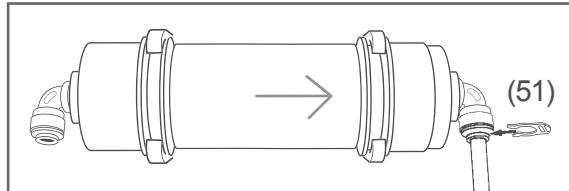
4. Fix the appliance hose in place using a safety clip (51).
