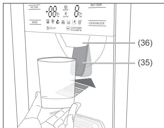
2. Hold the vessel as closely as possible to the opening for the ice (36), in order to avoid ice cubes from falling out around the sides of the vessel.
