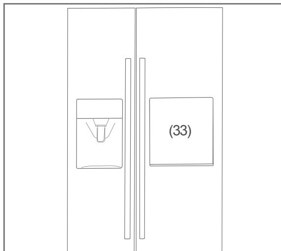
You can minimise the loss of refrigeration in the fridge by keeping frequently used bottles, drinks cartons, drinks cans, etc. in the bar compartment (33) in the door of the fridge compartment.
