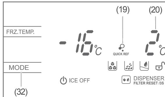
Select the (19) QUICK REF “Quick refrigerating” setting when you would like a can you have put in the fridge to be cooled faster, for example.
