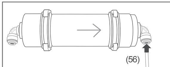
3. Insert the end of the appliance hose into the hose coupling to which the arrow on the water filter is pointing until it makes contact.
