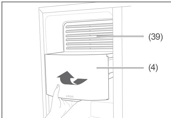
3. Lift the ice cube container slightly (4) and pull it out, keeping it level.
