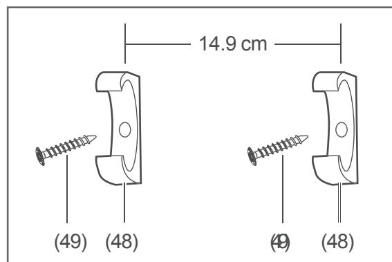
6. Screw the wall brackets (48) tightly onto the wall with the screws (49). Use the cross-tip screwdriver.
