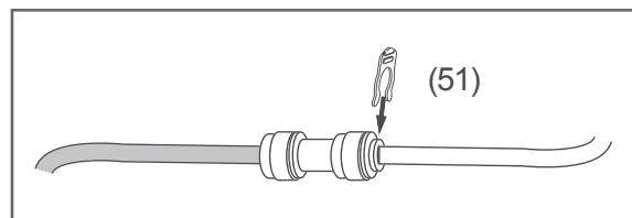
2. Fix the extension hose in place using a safety clip (51).
