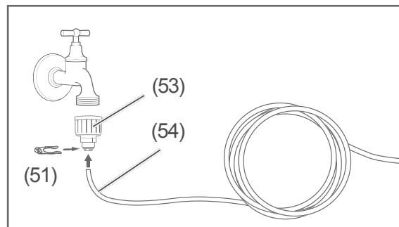
2. Push the inlet hose (54) into the  $\frac{3}{4}$ -inch screw connector (53) and affix the inlet hose with a safety clip (51).
