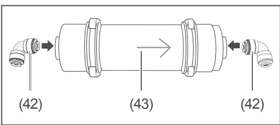
1. Insert the hose couplings (42) into the water filter (43) and firmly press them down.
