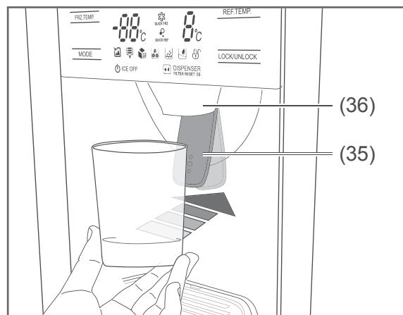
2. Hold the vessel as closely as possible to the opening for the ice (36), in order to avoid crushed ice from spraying out around the sides of the vessel.
