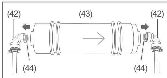
5. Loosen the connection between the hose coupling (42) and water filter (43). To do this, push the connector ring (44) on the hose coupling in the direction of the hose coupling using a small slot screwdriver while pulling off the hose coupling. Have a second person assist you if necessary.
