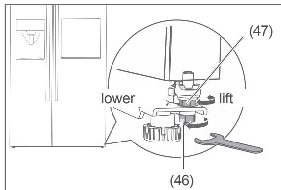
2. Turn the locknut (a) clockwise with two whole rotations to loosen it. Use the spanner supplied to do this.
