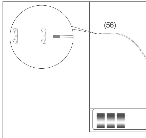
1. Determine the installation height of the water filter (43). The white appliance hose (56) must be able to reach the water filter. If the white appliance hose is too short, extend it by using the blue extension hose (57) (see "Extending the appliance hose" on page EN-40).
