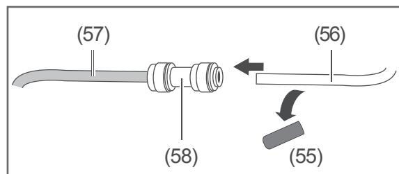
1. Remove the cap (55) from the white appliance hose (56) and insert the end of the appliance hose into the hose coupling (58) on the extension hose (57) until it makes contact.
