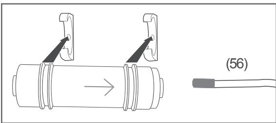
8. Press the water filter into the wall brackets so that the arrow on the water filter points in the direction of the white appliance hose (56).
