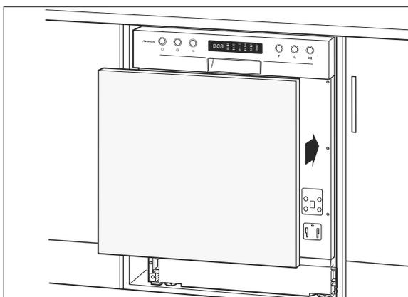
16. Fix the front panel to the dishwasher door using the Velcro straps (h), hold it firmly and carefully open the door.
