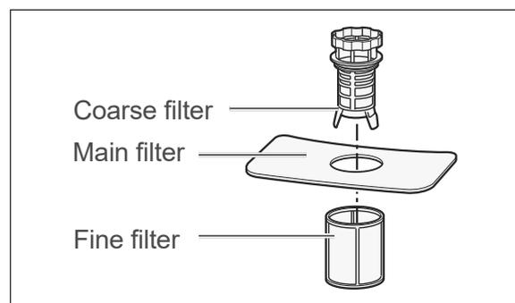
Check the coarse filter, the main filter and the fine filter after each rinse cycle and remove food residues and foreign bodies if necessary:
