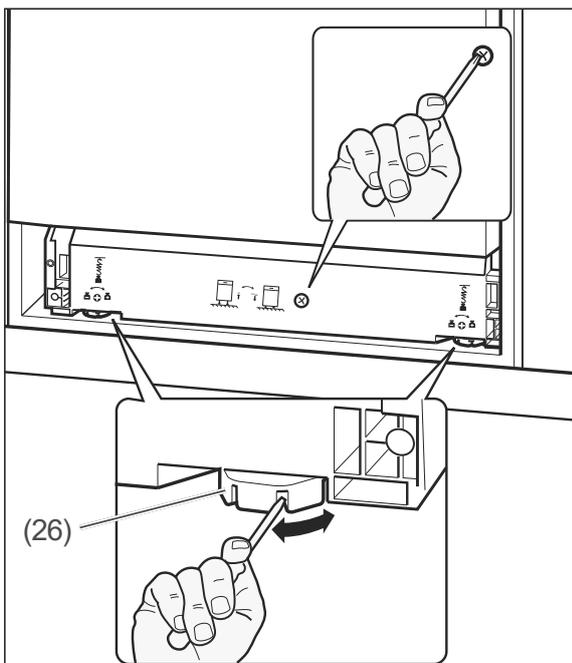
8. To enable the dishwasher to be positioned in a level position, both the front (26) and back appliance feet can be adjusted by up to 50 mm.
