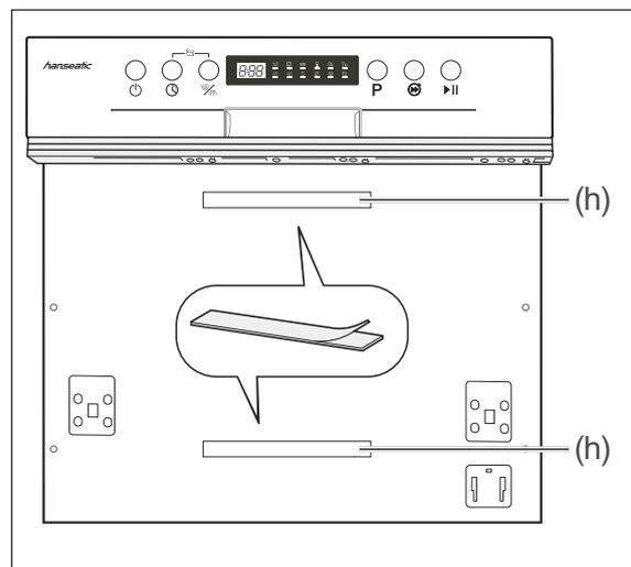
9. With the protective film removed, stick the Velcro straps (h) to the middle of the recessed areas on the dishwasher door.
