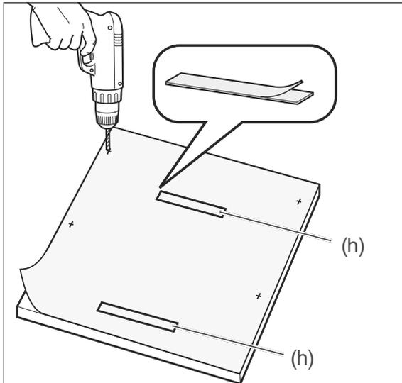
12. Lay the enclosed drilling template on the **back** of the front panel in such a way that the drilling template and the front panel are flush at the top.
