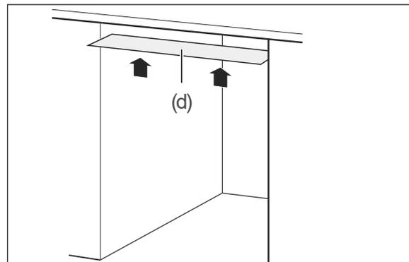
3. Affix the condensation protection film supplied (d) to the underside of the worktop. In this way, you will avoid damage to the work surface as a result of hot steam which may be emitted from the dishwasher if the dishwasher door is left open.
